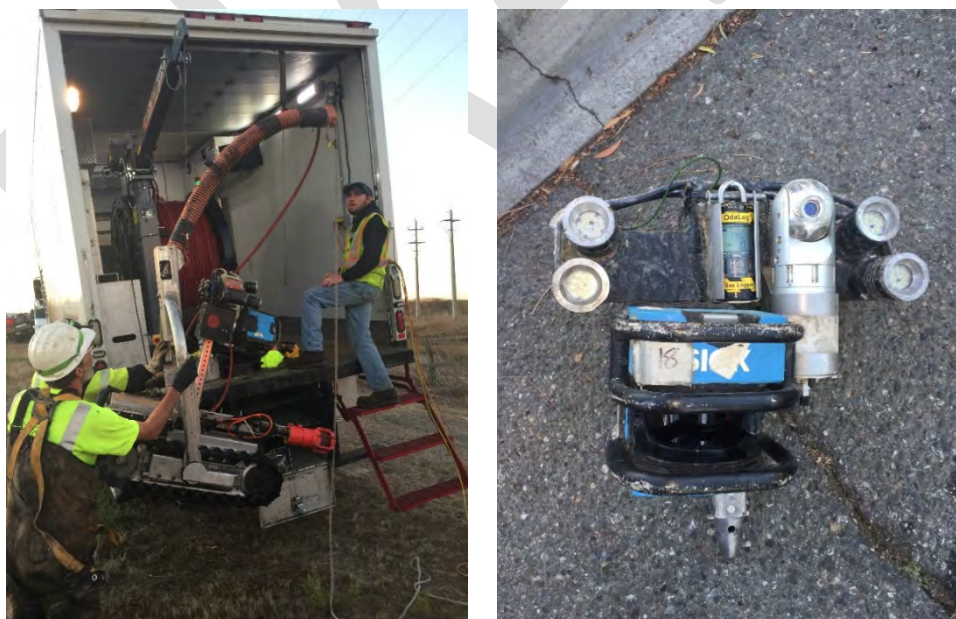
Figure ES-3. RedZone Responder platform (left) and mast with lights, CCTV, LiDAR and sensors (right)
