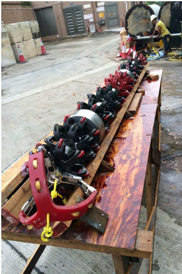
Photo 1.17: PICA Seesnake Internal Pressure Main Inspection Tool
